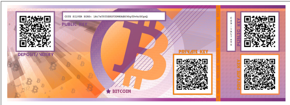
Figure 4-12. An example of a paper wallet with additional copies of the keys on a backup “stub”
