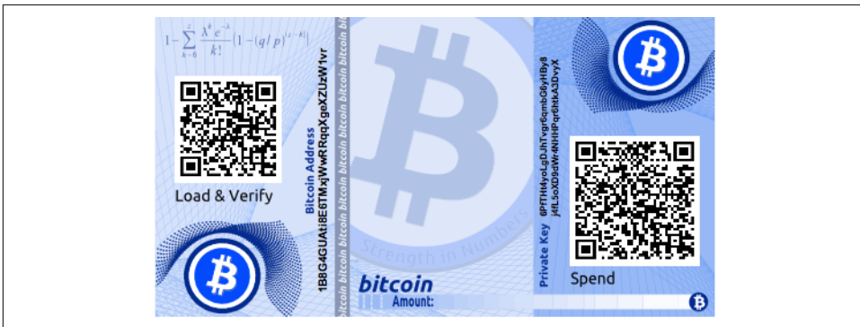
Figure 4-9. An example of an encrypted paper wallet from bitaddress.org. The passphrase is “test.”
